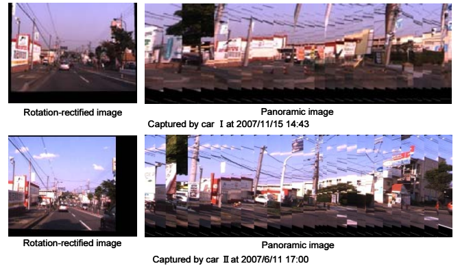
Fig. 14. Rotation-rectified image and a generated panoramic image.
